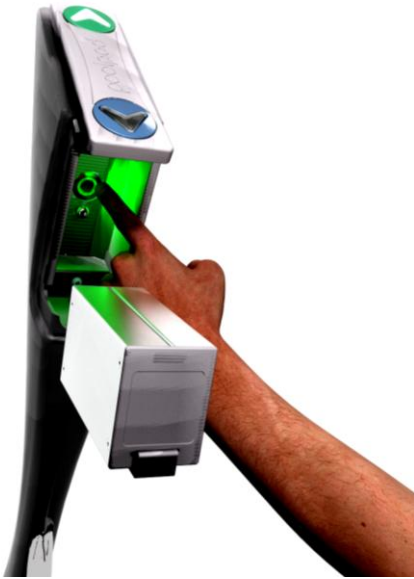
c. Tap the power button located inside the battery holder and this will illuminate green.
